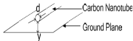
Fig.2. Isolated conductor, with diameter ‘ d ’, over a ground plane at a distance ‘ y ’ below it.
